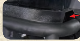
Textured plastic filler plate fills in the gap between the body and the bumper, a Rugged Ridge® exclusive.
