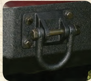
D-rings attach securely to the frame of the vehicle for a rock solid recovery mounting point.
