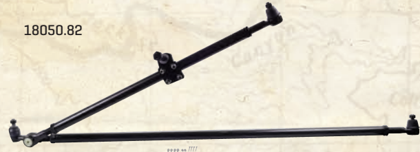
Heavy Duty Crossover steering systems prevent "bump steer"!
