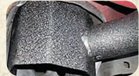
07-12 Wrangler models have simple bolt on design. Utilizes existing body mount locations on frame.
