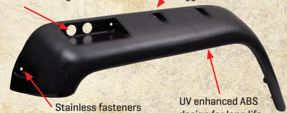
Custom designed for use with the factory side marker light
