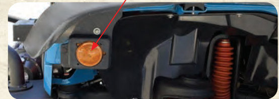
Special side marker light brackets included for use with your factory side marker light
