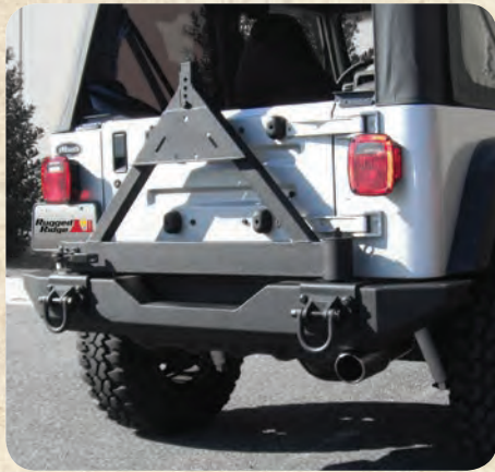
D-rings attach securely to the frame of the vehicle for a rock solid recovery mounting point.
